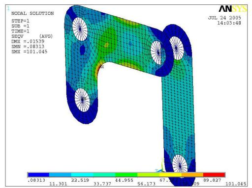
3. A contour plot of the von Mises stress should produce the following plot:
