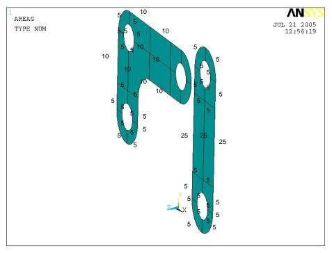
Figure 4. Divisions Applied to Lines for Mesh Control
