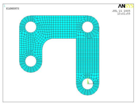
Figure 5. Mesh of the Plate Midsurfaces
