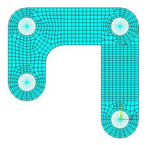
Figure 6. Mesh Including MPC's at the Holes
