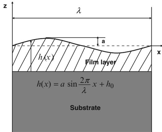
**Fig. 1** Schematic illustration of sinusoidal strained film on a flat substrate
