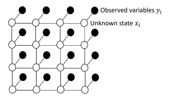
In a simple depth estimation problem on an image of size 1000 x 1000, every node can have states from 1 to D denoting different distances from the camera center.
