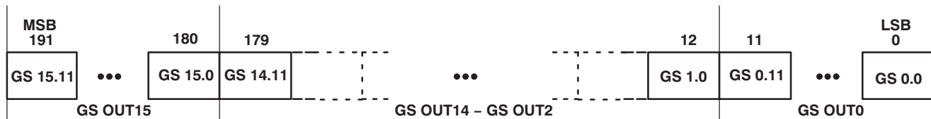
Figure 18. Grayscale Data Packet Format
