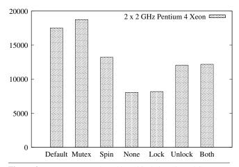
Figure 4. Msecs to copy 10MB/thread in 2 threads on 2GHz Pentium 4 Xeon
