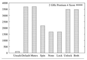
Figure 2. Msecs to copy 10MB on 2GHz Pentium 4 Xeon
