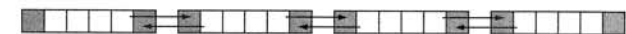
Figure 4.10: A data distribution with ghost boundaries. Shaded cells are ghost copies; arrows point from primary copies to corresponding secondary copies.
