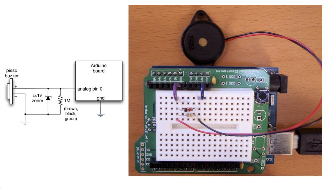
Create two little busses for GND and A0, and hook components across it. Black bar on diode indicates "bar" of diode.
