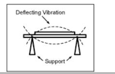
Oscillating voltage alternately squeezes and releases the piezo element. Must apply flucuating voltage, a steady HIGH or LOW won't work.
