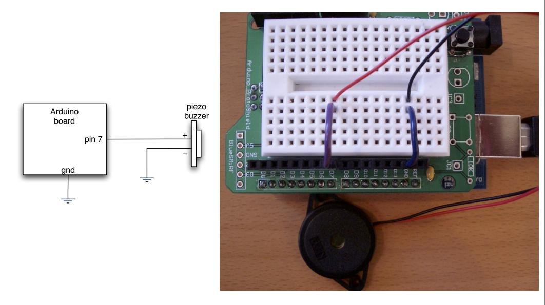
Piezo leads are very thin. The breadboard holes grab them better than the header sockets, which is why the jumper leads are used.
