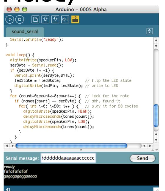
This sketch is in the handout, and is based on "Examples/pwm\_sound/keyboard\_serial" Notice the problem with this sketch? Different notes play for different amounts of time. 50 cycles of low C isn't the same amount of time as 50 cycles of high B
