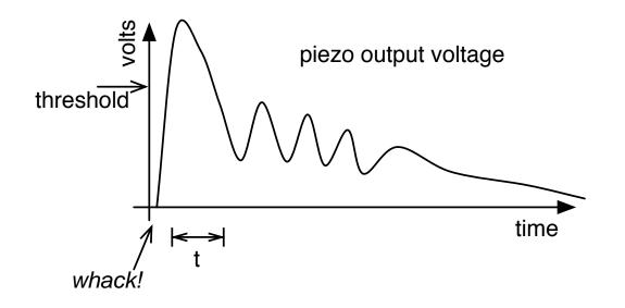
Depending on how fast you can watch the input, this technique works either really well or not that well. There are much faster ways of watching inputs that loops with analogRead() But for now it works okay
