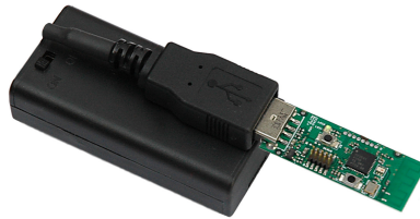
FIGURE 2. TI CC2531 “USB dongle” nodes used in experimental tests.
