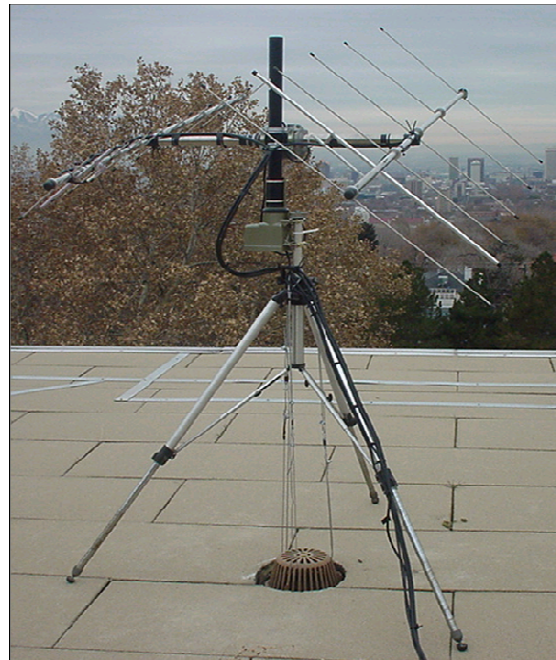
Figure 1: Antenna array mounted on a tripod with azimuth and elevation control rotators
