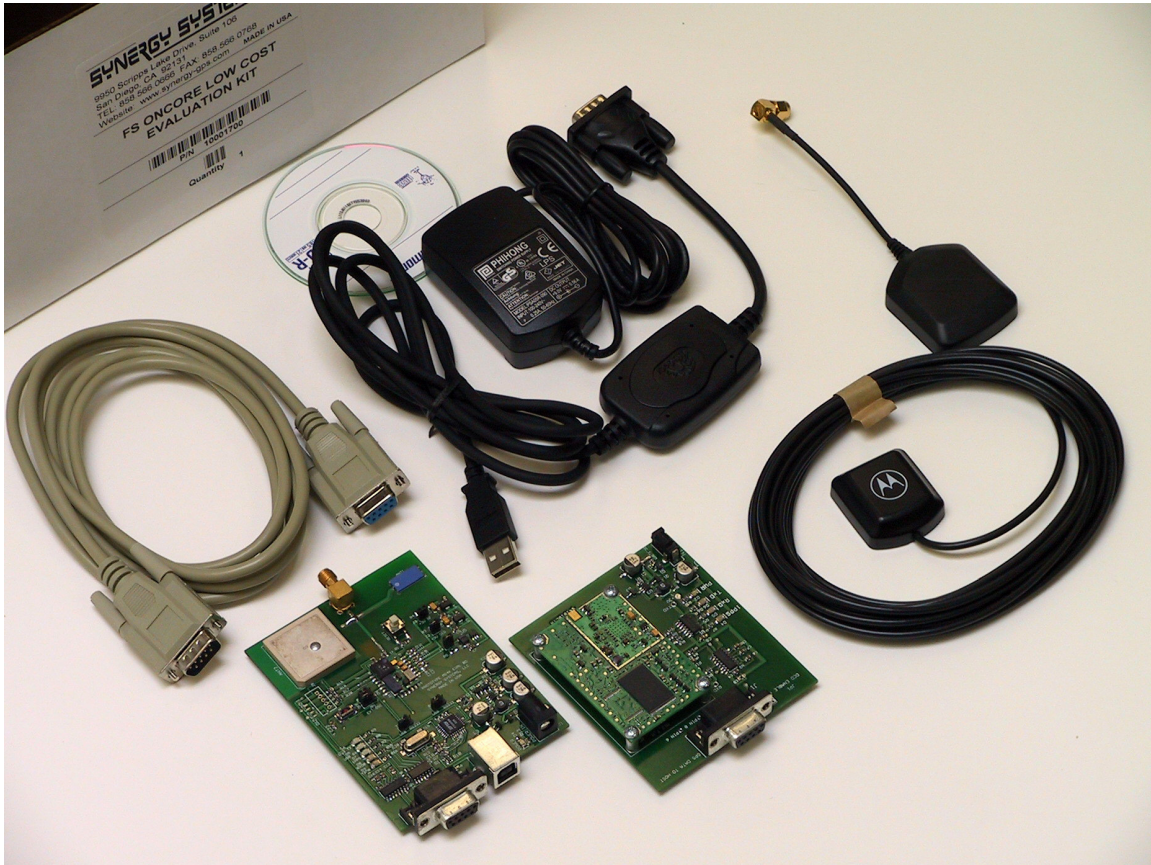
(See Motorola's Semiconductor Technical Data, Evaluation Tools – Preliminary for the Low Cost Evaluation Kit for the FS Oncore GPS Module)
