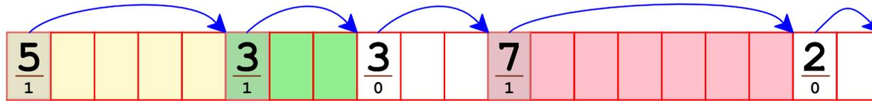
How does the allocator know that the size-2 block is the last one?
