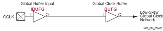
a. Global Buffer Inputs and Clock Buffers Drive a Low-Skew Global Network in the FPGA
