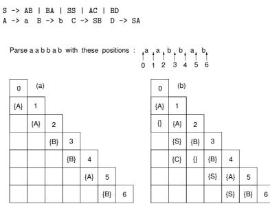
Fig. 14.8. Steps of the CKY parsing algorithm on input aabbab
