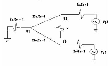
Split down the center, so that the output ports will act on the circuit separately. This will ensure complete isolation later.
