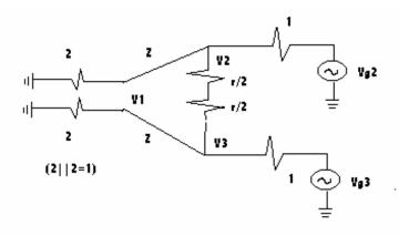
S-parameters:  $S32 = V_3^- / V_2^+$  when  $V_3^+ = 0$ .
