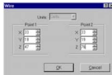
Figure 62: The Wire primitive data for the monopole.
