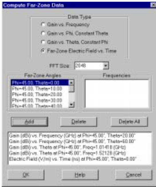
Figure 51: The Compute Far-Zone Data window for a Transient Far-Zone calculation.
