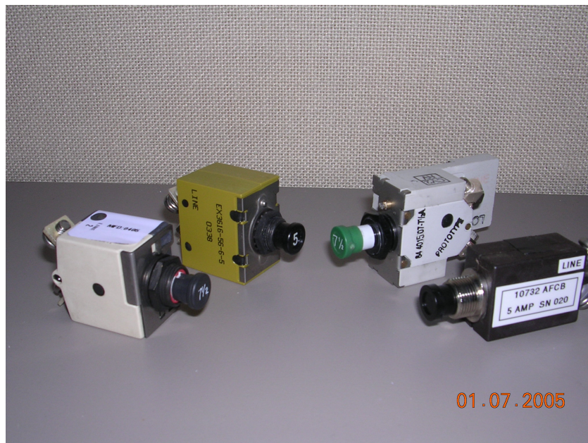
Figure 8. Arc Fault Circuit Breakers.
