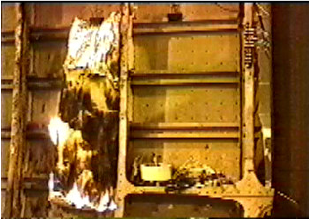
Figure 6. Insufab™ 350 Type K Arc Damage (Large open flame/both sides of film consumed).
