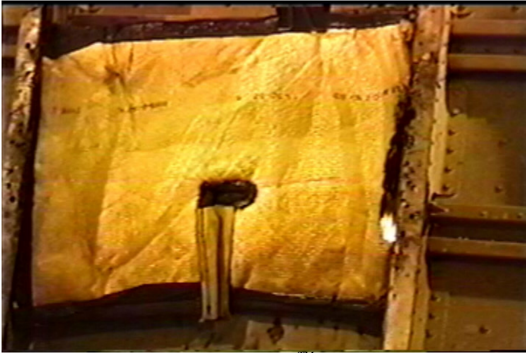
Figure 5. Plain Mylar™ 1.5 PCF Arc Damage (Only the edge damaged).
