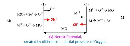
The above figure shows that for every one  $O^{-2}$  ion moving,  $2h^+$  move in the same direction; and for every one  $M^{+2}$  moving,  $2e^-$  move in the same direction.
