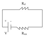
The internal current density,  $I_{int} = \frac{V}{R_{ion} + R_{el}}$ , where V is the Nernst potential
