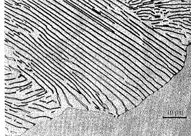
FIGURE 5.60 Pearlite colony advancing into an austenite grain. (After Darken, L.S. and Fisher, R.M., in Decomposition of Austenite by Diffusional Processes , Interscience, New York, 1962.)
