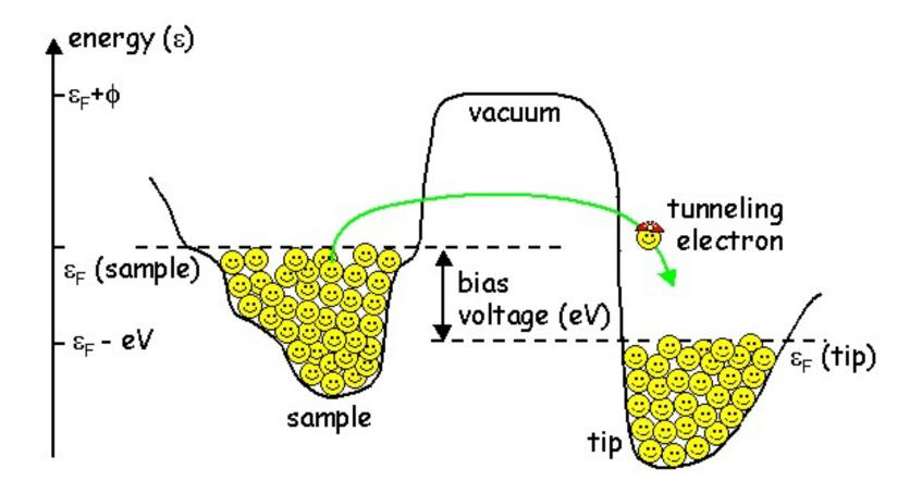
By applying a bias voltage to the sample with respect to the tip, we effectively raise the Fermi level of the sample with respect to the tip. Now we have empty states available for tunneling into.
