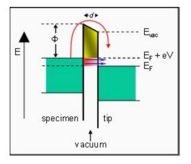
If the distance d between specimen and tip is small enough, electrons can 'tunnel' through the vacuum barrier. When a voltage V is applied between specimen and tip, the tunneling effect results in a net electron current. In this example from specimen to tip. This is the tunneling current.
