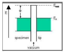
When the specimen and the tip are brought close to each other, there is only a narrow region of empty space left between them. On either side, the electrons are present up to the Fermi energy. They need to overcome a barrier  $\Phi$  to travel from tip to specimen or vice versa.
