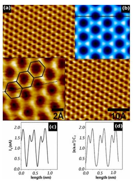
(a) (Color online) Experimental STM image of HOPG at constant-height mode, Vb=–300 mV. (b) Calculated STM image at constant-height mode, Vb=–300 mV, and tip surface distance of 1.2 Å. Both images reveal the hexagonal atomic structure which is compound by  $\alpha$  and  $\beta$  atoms. (c) And (d) are line profiles along the lines indicated in (a) and (b), respectively.
