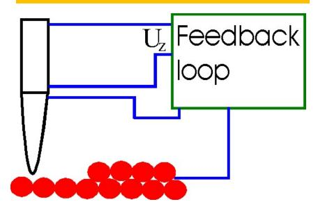
Imaging the surface topography at atomic resolution if the surface is composed of the same atoms, *i.e., the only factor affecting the tunneling current is the distance.*
