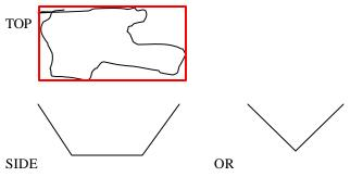
4. Draw the etch profile for the mask opening below for both an isotropic and anisotropic (crystal dependent) silicon etch assuming that the etch is allowed to continue until it just reaches the bottom edge of the substrate.
