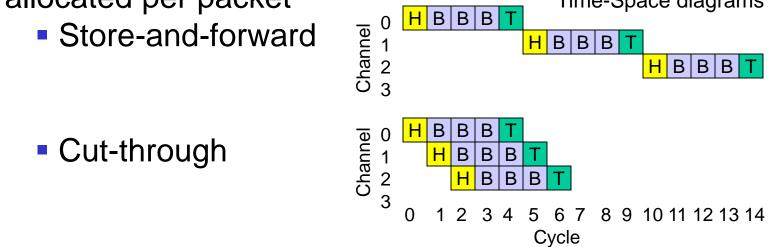
Wormhole routing: same as cut-through, but buffers in each router are allocated on a per-flit basis, not per-packet
