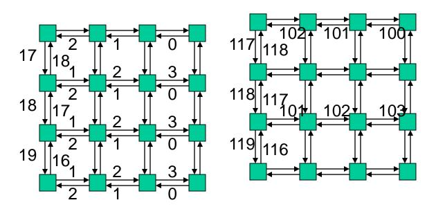
Alternatively, use West-first routing on the 1<sup>st</sup> plane and cross over to the 2<sup>nd</sup> plane in case you need to go West again (the 2<sup>nd</sup> plane uses North-last, for example)
