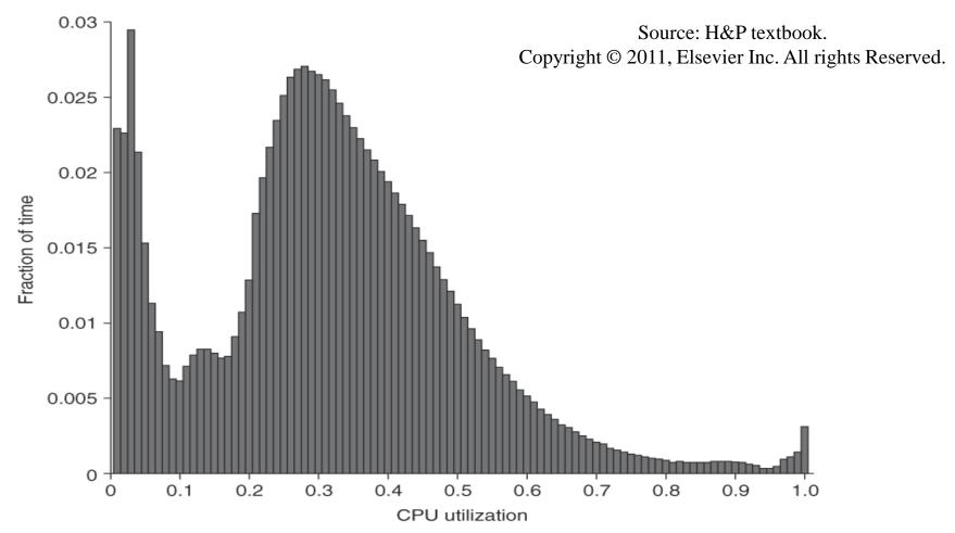
**Figure 6.3** Average CPU utilization of more than 5000 servers during a 6-month period at Google. Servers are rarely completely idle or fully utilized, in-stead operating most of the time at between 10% and 50% of their maximum utilization. (From Figure 1 in Barroso and Hölzle [2007].) The column the third from the right in Figure 6.4 calculates percentages plus or minus 5% to come up with the weightings; thus, 1.2% for the 90% row means that 1.2% of servers were between 85% and 95% utilized.
