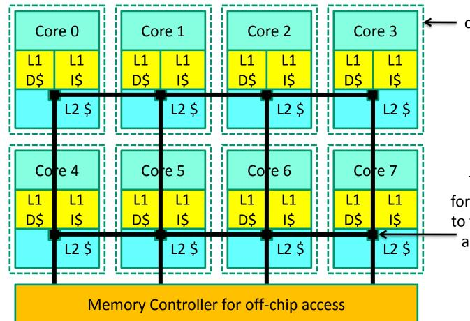
A single tile composed of a core, L1 caches, and a bank (slice) of the shared L2 cache
